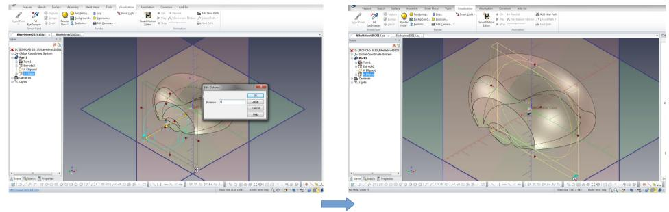
Change View to Front and use the TriBall to copy the H Ellipse to left, and re-size the Height/Depth of the copied feature.
