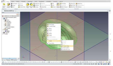
Select View > Rotate and select the outer edge Part1 and set blend
