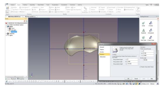
Position the H Ellipsoid as the right head cavity.
