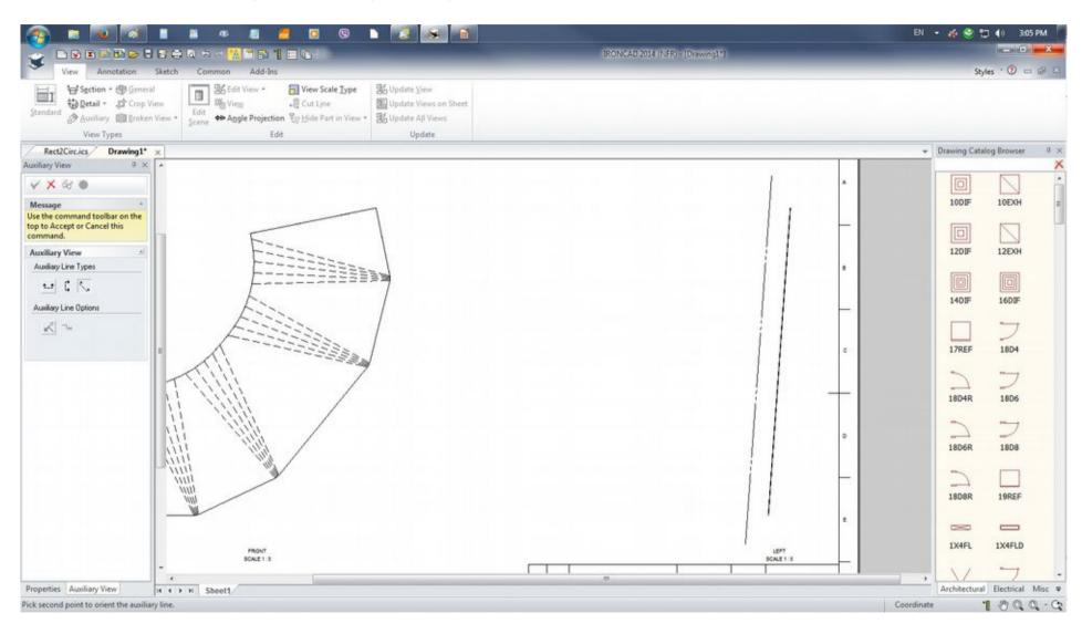
Drag and position the displayed sectional line in place with LMB click. Please note the direction of the line end arrows. It can be switch by the Auxiliary Line Options. Click the Check button to create. Place and LMB click the view outline in place and hit the Esc button to release. The Auxiliary A-A view project the true flat pattern showing the bend lines and manufacturing string.
