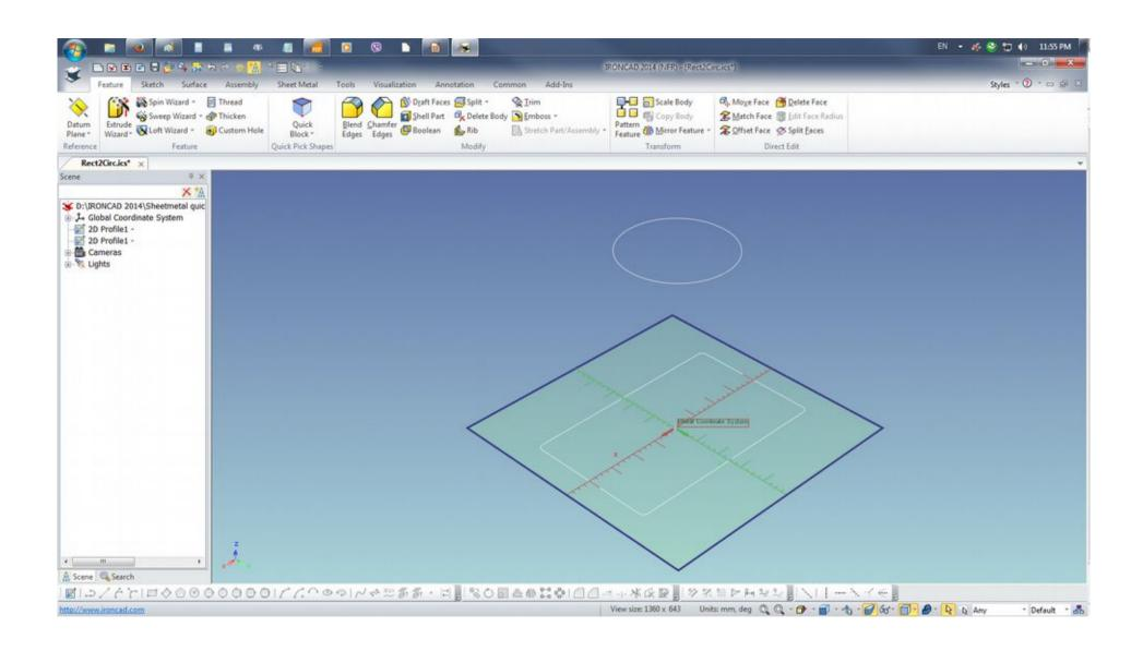
Go to the Sheet Metal tab and select Create Loft operation. Select the profiles for the section and Change Stock to the desired material.
