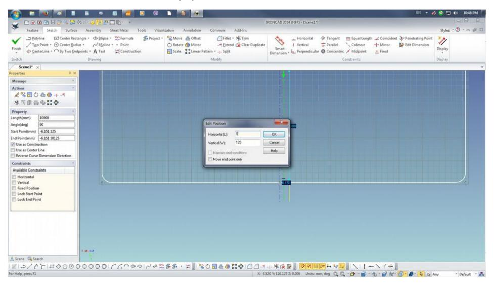
Point the cursor on the point of the construction line intersection on drawing grid an use the scroll will to zoom in or out. Select Trim Curve and point the cursor between the construction line. Notice the green broken line that will create the split or gap between construction lines. Once the gap is created click Finish
