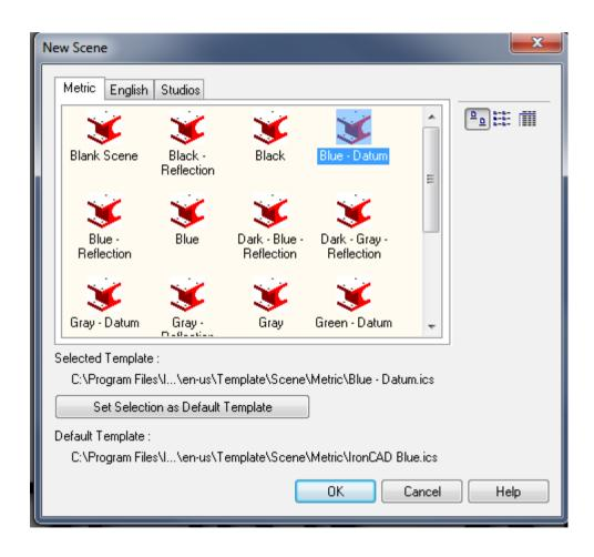
The Datum Screen is used so you will be aware of the 0,0,0 position that can be of value when creating items to used in a catalog or assembly. Press keys X, Y to hide YZ and XZ planes.
