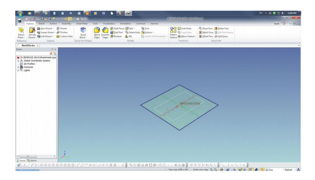
Select 2D Profile1 > key F10 to activate TriBall and point cursor on the top vertical handle and depress RMB and drag upwards. On release select Copy and enter 350 on the Distance field of the Repeated Copy / Link dialogue box.
