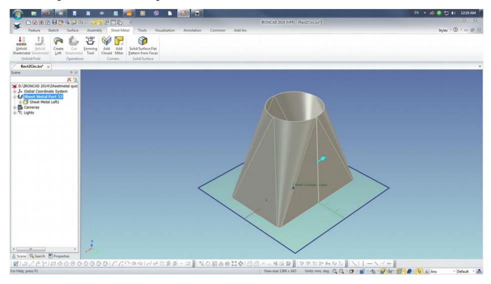
To perform a bend line check or if the created Sheet Metal Loft was done with the values set, select Solid/Surface Flat Pattern from Faces. Select this face as it registers to Face Selection box and click the Check mark.
