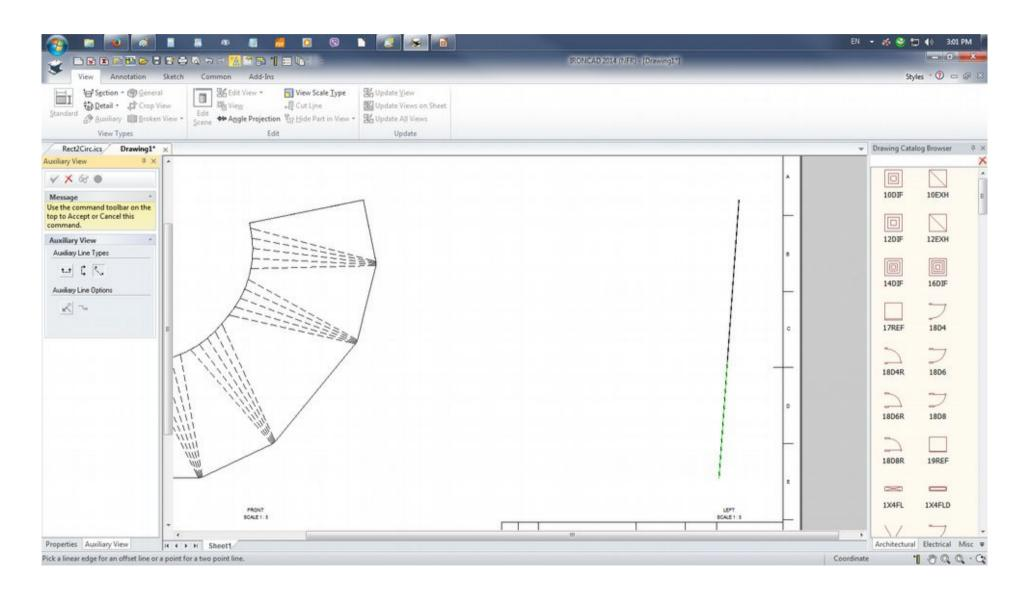
Drag and position the displayed sectional line in place with LMB click. Please note the direction of the line end arrows. It can be switch by the Auxiliary Line Options.
