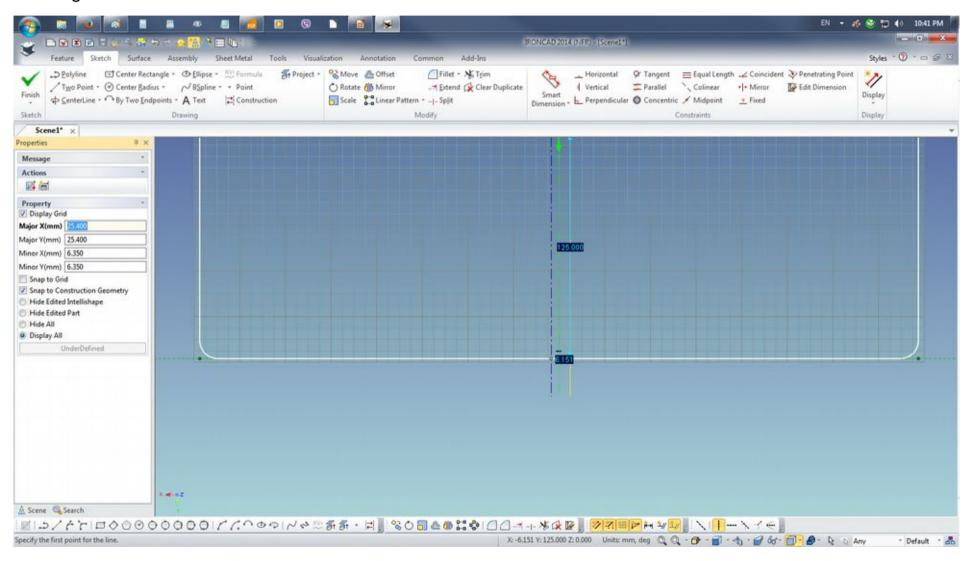
Point cursor on the horizontal value and perform RMB click to edit the value and enter 1. Perform on the same edit on the other vertical construction line. Please note the Show Curve Dimensions and Show Endpoint Dimensions show be activated from Display button to show.
