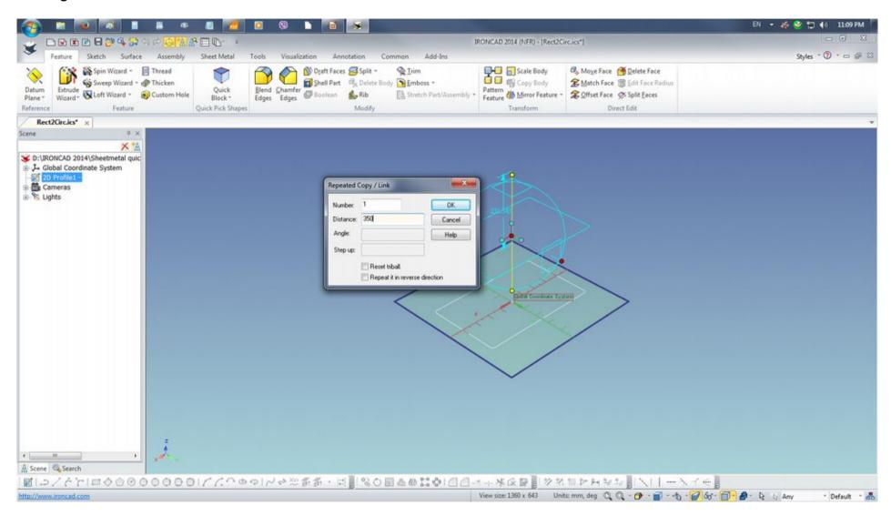
RMB click to select and Edit the copied 2D Profile1. Draw a Center Rectangle from the center of the drawing with RMB drag and on the Edit Rectangle dialogue box. Enter 200 for both fields and click OK. Press Esc to release previous selected tool. Click on the previous drawn rectangular box to delete.
