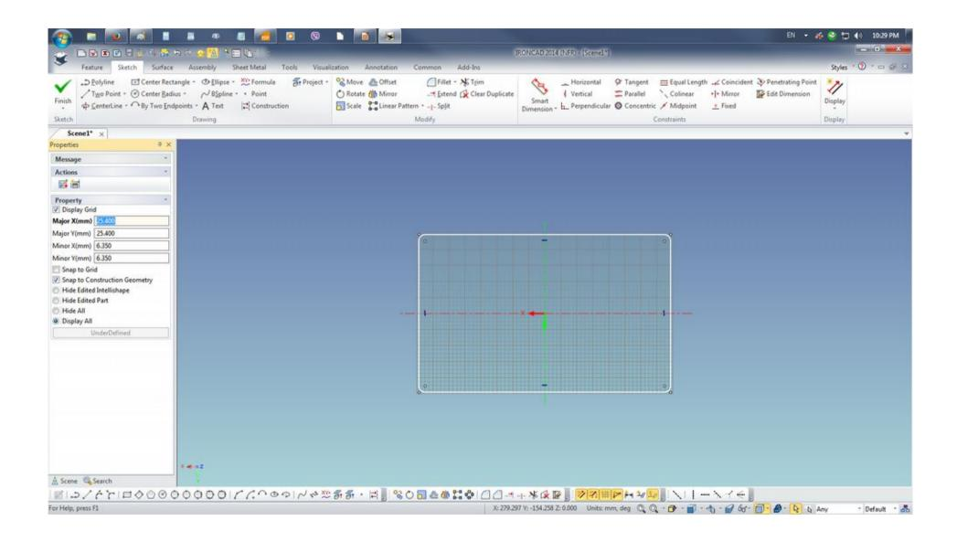
Next a split/gap must be created on the rectangular sketch so it work with the Create Loft on the Sheet Metal operation later. The split or gap can be created by drawing a small Center Rectangle or Center Radius Circle drawing on a center point on the location of the split or gap and using the Trim Curve to create the break on the rectangle. I tend to use the construction line as a force of habit as it records on the edit of the section.
