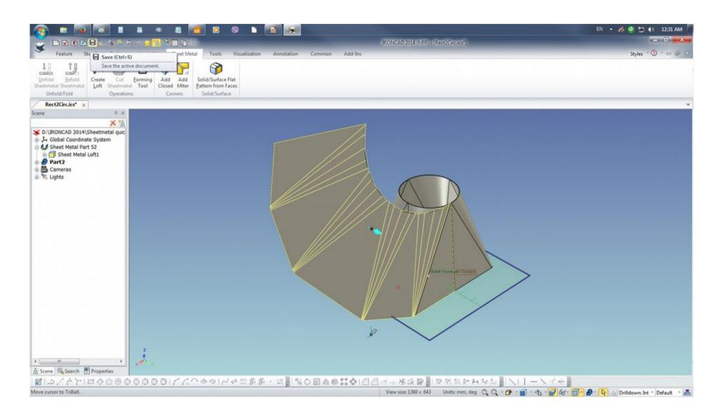
Delete the created Part 2 and select the Sheet Metal part and select Unfold button or on the RMB click select Unfold
