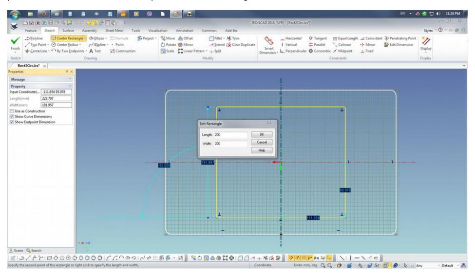
Zoom in to split/gap point. As the Vertical Construction Line is still in place, perform the Trim Curve command to create the split/gap between the construction lines
