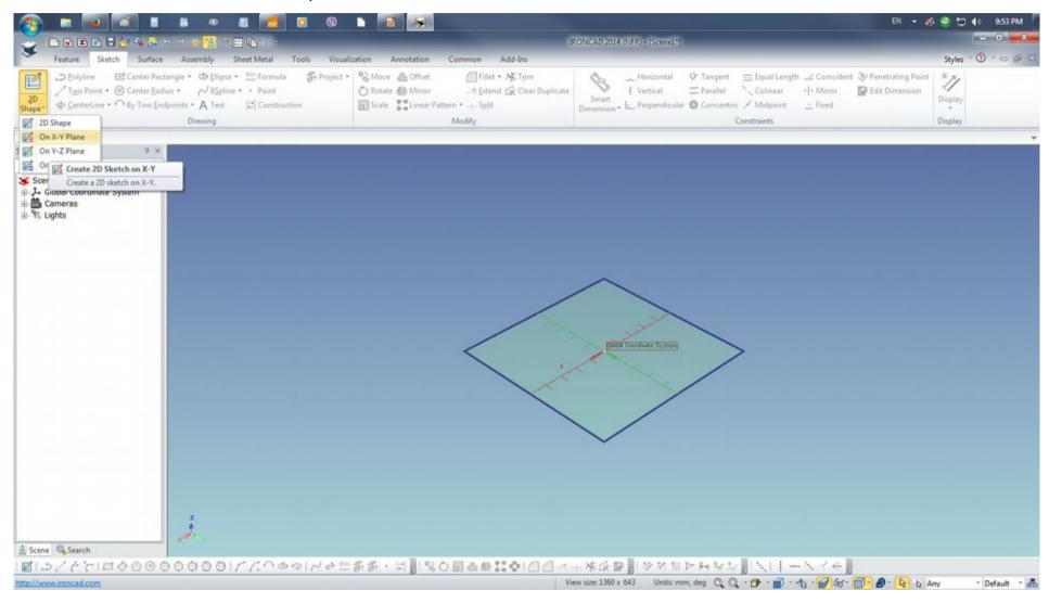
From the drawing tools, select Rectangle on the drop down list, select Center Rectangle. Point cursor at the center of the drawing grid. Depress the RMB and drag to draw the rectangle and tupe the values as shown on the Edit Rectangle dialogue box and click OK to confirm action.
