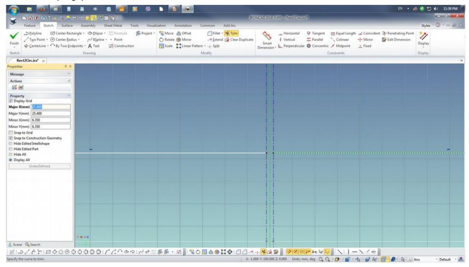
Press F8 (Fit Scene) to view. Select Fillet and point the cursor on bottom left side corner with a split horizontal line. Depress RMB and drag the corner Fillet towards the center of the drawing grid to get the maximum value and edit to 98.4. Perform all the Fillet with same action and enter the same value on three other corners to create a consistent symmetrical corner blends and Click Finish to end the edit on the section.
