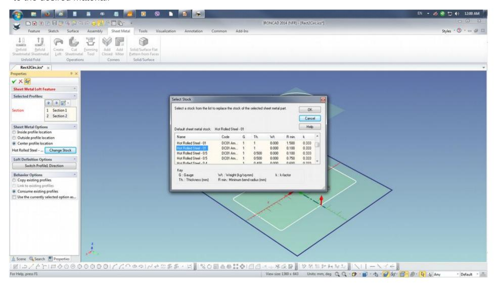
If it fails to generate a preview, Switch Profile1 Direction from the Loft Definition Options to generate.
