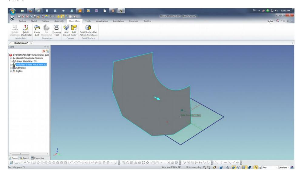
To create the IRONCAD Drawing (ICD) on File > New > Drawing and select the appropriate Template sheet.
