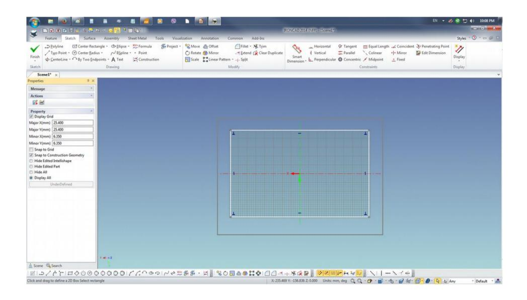
Click on Fillet tool from the Modify tool set. Pick corner and depress the RMB and drag. Upon release of the RMB fill the value of 10 on the Edit Radius dialogue box and click OK
