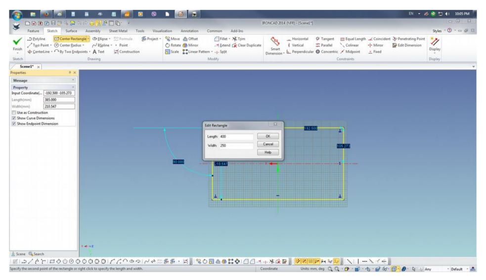
Depress the LMB to select with cursor the drawn rectangle to highlight the object. This will facilitate the Fillet to be done in all corners of the rectangle.
